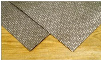
ME-2100 is a simple solution for effective RF signal attenuation in many commercial applications. It provides -100 dB RF isolation from 100 MHz to 1 GHz and more than -70 dB to 18GHz. Very light, thin, flexible, wear and tear resistant, it can be applied directly to studs, standard sheetrock and other structures using simple and inexpensive methods. The product is well suited to both new and retrofit construction. It provides a good degree of
